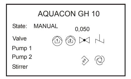
During manual operation, the pump, the sample inlet valve and the stirrer can be activated/deactived by touching the appropriate symbols. The active part will be displayed with inverse letters.
