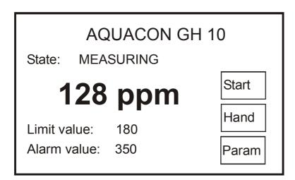
The automatic analysis cycle can be interrupted at any stage by touching the button "Hand" or the button "Param" on the touchscreen (see chapter 3.5).
