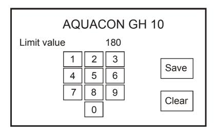
To leave the screen and confirm/safe the new parameter value, the button "Save" must be touched. To leave the screen without saving, the button "Clear" must be touched.
